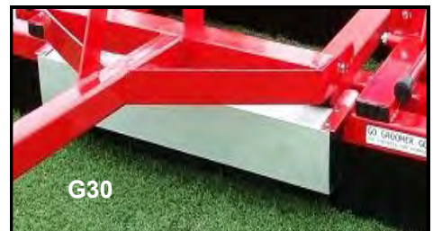
One G30 In-Line Safety Magnet mounted on front brush channel during grooming (more than one G30 In-Line Safety Magnet can be used while grooming)
